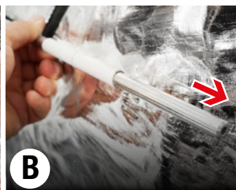
2.) Push the rod extensions to the front and connect them to the other rod-end.
